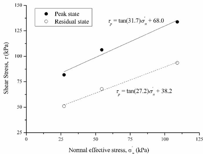
**Figure 9 Mohr-Coulomb failure envelope of the compacted CKLS from TP-1**
