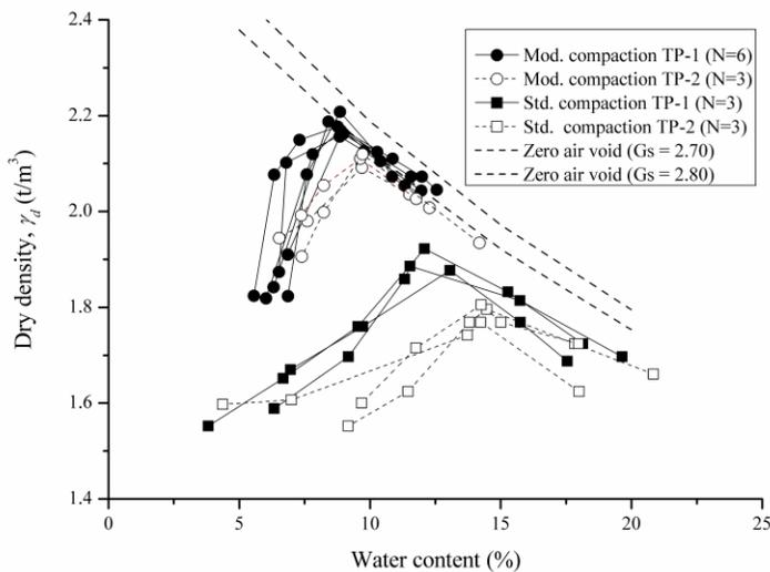
**Figure 5 Results of modify and standard compaction test**
