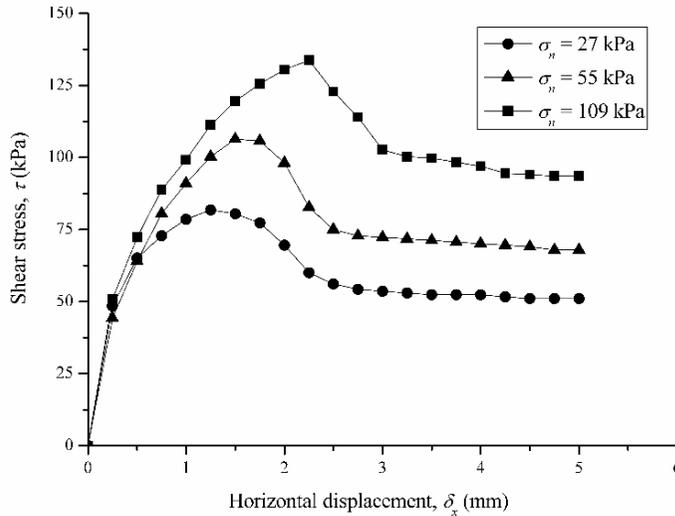
**Figure 8 The test results of the shear stress-displacement of the compacted CKLS from TP-1**
