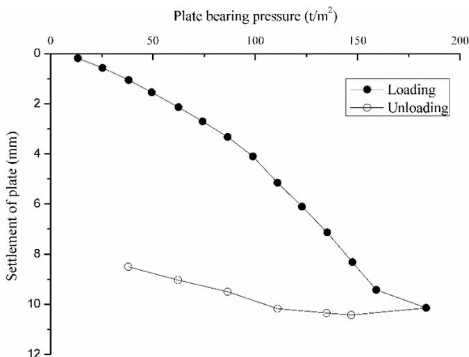
Figure 11 Test results of plate bearing
