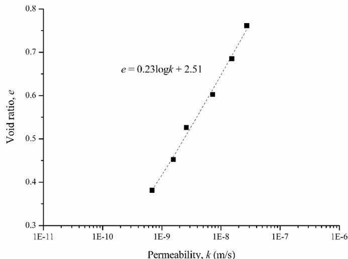
**Figure 10 Relationship between void ratio ( $e$ ) and  $\log k$  of CKLS**
