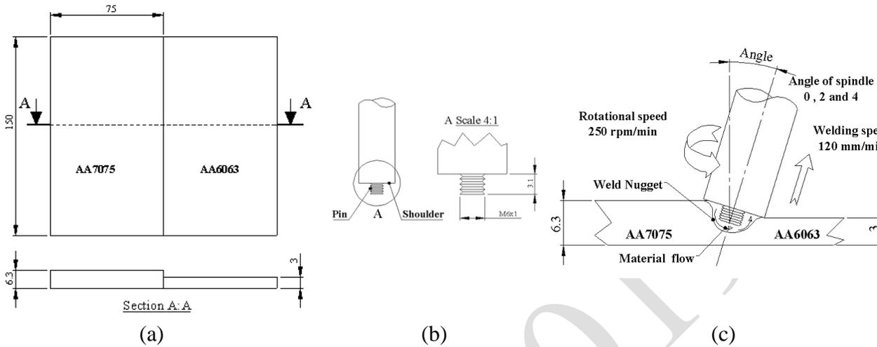
**Figure 3 Characteristics of TWBs aluminum alloy sheet by FSW joints. (a) Workpiece position (b) Tool geometry (c) Welding process**
