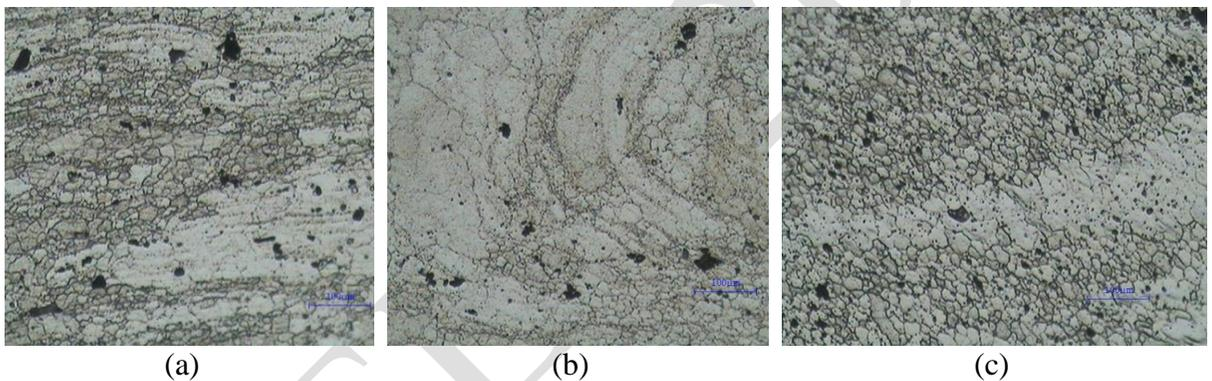
**Figure 5 Characteristics of microstructure TWBs aluminum alloy sheet by FSW. (a) 250 rpm/min (b) 500 rpm/min (c) 1,000 rpm/min**
