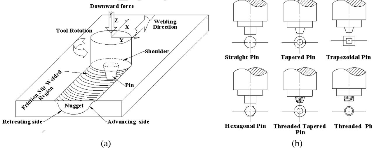
**Figure 1** The friction stir welding occurred in (a) friction stir welding process. (b) Schematic drawing of the FSW tool geometries [11]
