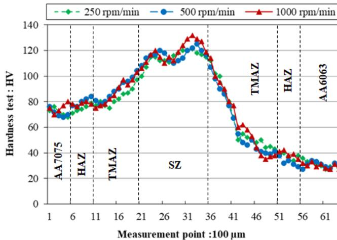
Figure 6 Hardness profile across the weld joint along.
