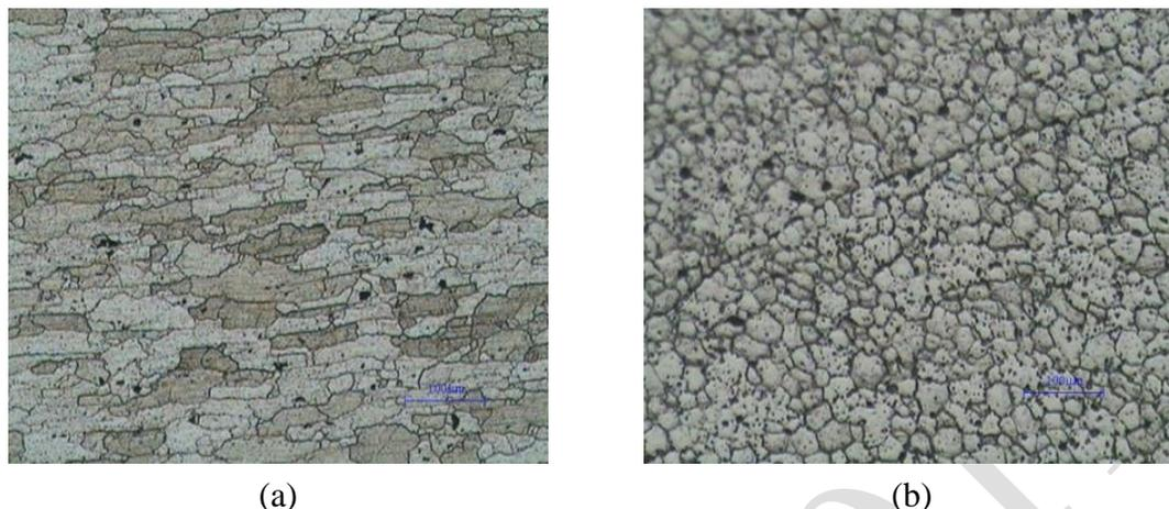
**Figure 2 The microstructure of base material in the experimental. (a) AA6063 aluminium alloy (b) AA7075 aluminium alloy**
